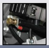
Battery: "Extended" battery pole allows the battery to be recharged without having to open the battery box.
