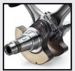
Crankshaft: Forged, one-piece crankshaft. 125 mm forged con rod. Stroke 62.4 mm, adapted to the bigger displacement of the 999cc engine.
