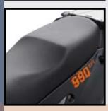
Seat: The S-model is fitted with a more offroad-oriented seat. Seat height 895 mm. The 990 Adventure with a lower seat and a stepped contour, seat height 860 mm.
