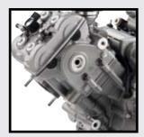
Cylinder: New cylinders with bore of 101 mm.
