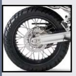
Wheels: 18/21" wheels ideal for off- and onroad use. The front wheel with an improved and more stable 2.15" rim. Large range of offroad tyres available. For offroad KTM recommends new Continental TKC 80 specially developed for KTM.
