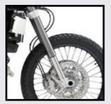
Braking System: New floating brake discs and relocation of the front steelflex brake lines.
