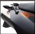
Silencer: Two stainless steel silencers, each with three-way catalytic converter.
