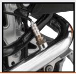
Lambda sensors: One Lambda sensor per cylinder feeds back information on the emissions to ECU.
